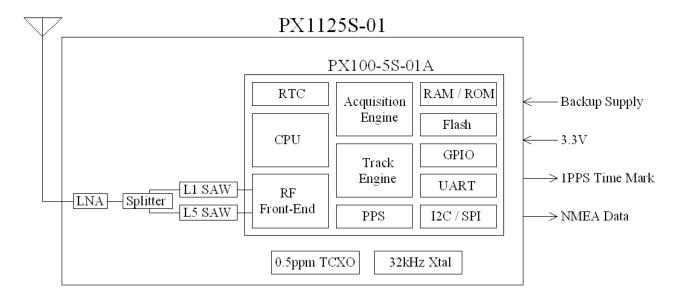
The PX1125S-01 is a L5 NavIC + L1 GAGAN/GPS satellite navigation receiver in a compact surface mount package. It is based on the latest single-chip Phoenix GNSS receiver technology, providing high performance signal acquisition and tracking. The simple UART serial interface and the standard NMEA-0183 protocol make usage of PX1125S-01 very easy and straightforward.
