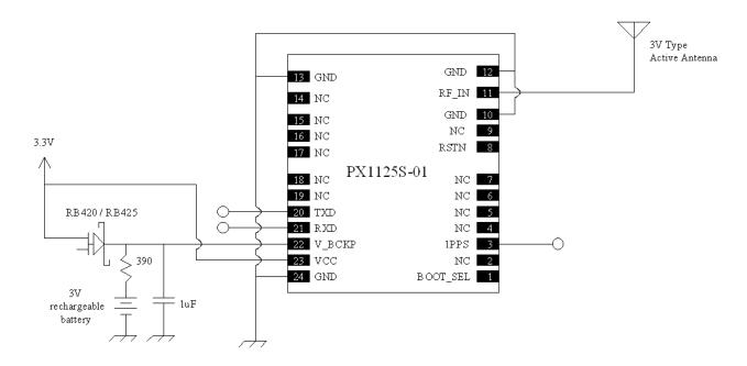
When PX1125S-01 has previously been used within 2 hour, for faster time to first fix powering up without needing to decoded ephemeris data from signal, V\_BCKP should be connected to non-volatile supply; above figure with V\_BCKP connected to rechargeable battery is an example implementation. If cold starting every time powering up is not an issue, V BCKP can be connect to VCC.
